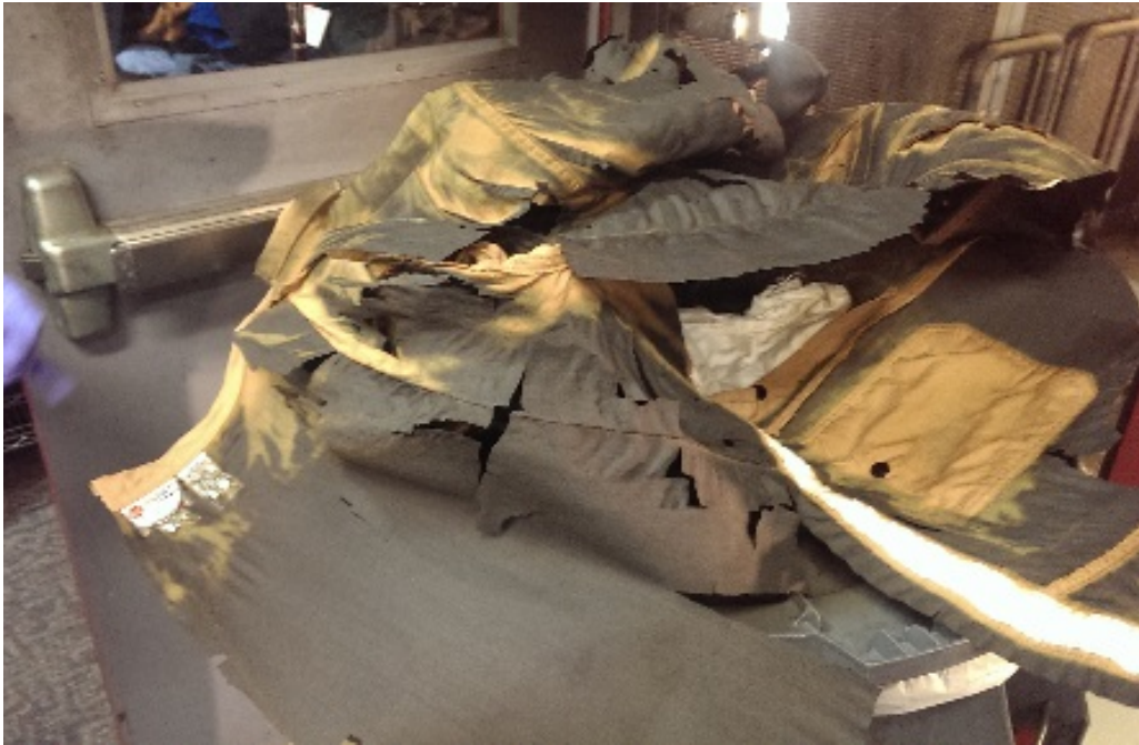
Example of FR garment that became brittle and broke open on the mannequin during a burn test
